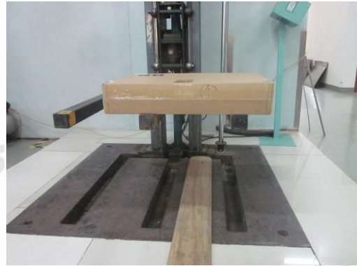
Face Drop on hazard
